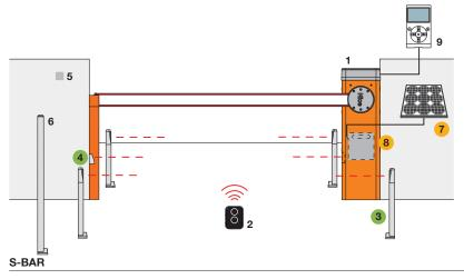
Motor 2. Transmitter 3. Photocells mounted on posts 4. Photocells 5. Digital or key switches 6. Key-operated selector or digital on post 7. SYP solar panel 8. PSY24 battery box 9. O-View multifunction display
