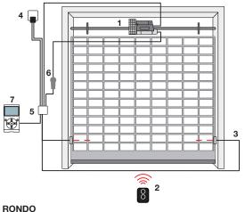
1. Motor 2. Transmitter 3. Photocells 4. Flashing light 5. Control unit 6. Digital or key switches 7. O-View multifunction display
