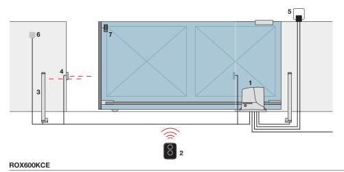
1. Motor 2. Transmitter 3. Photocells mounted on posts 4. Photocells 5. Flashing light 6. Key switch 7. Sensitive edges
