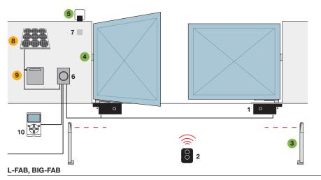
Motor 2. Transmitter 3. Photocells mounted on posts 4. Photocells 5. Flashing light 6. Control unit 7. Digital or key switch 8. SYP solar panel 9. PSY24 battery box 10. O-View multifunction display
