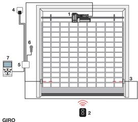
1. Motor 2. Transmitter 3. Photocells 4. Flashing light 5. Control unit 6. Digital or key switches 7. O-View multifunction display
