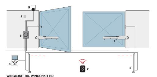
1. Motor 2. Transmitter 3. Photocells mounted on posts 4. Photocells 5. Flashing light 6. Control unit 7. Digital or key switch 8. O-View multifunction display
