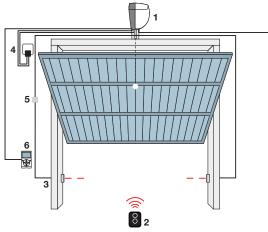
1. Motor 2. Transmitter 3. Photocells 4. Flashing light 5. Digital or key switches 6. O-View multifunction display
