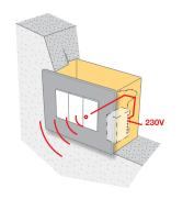
Recessed transmitters, **model TTX4** with mains power supply, and **TTXB4**, battery-powered.
