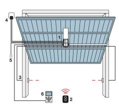
1. Motor 2. Transmitter 3. Photocells 4. Flashing light 5. Digital or key switches 6. O-View multifunction display
