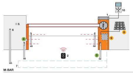
Motor 2. Transmitter 3. Photocells mounted on posts 4. Photocells 5. Digital or key switches 6. Key-operated selector or digital on post 7. Loop detector 8. SYP solar panel 9. PSY24 battery box 10. O-View multifunction display
