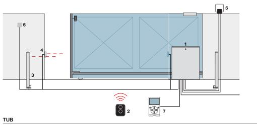
1. Motor 2. Transmitter 3. Photocells mounted on posts 4. Photocells 5. Flashing light 6. Key switch 7. O-View multifunction display
