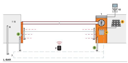
Motor 2. Transmitter 3. Photocells mounted on posts 4. Photocells 5. Digital or key switches 6. Key-operated selector or digital on post 7. Loop detector 8. SYP solar panel 9. PSY24 battery box 10. O-View multifunction display
