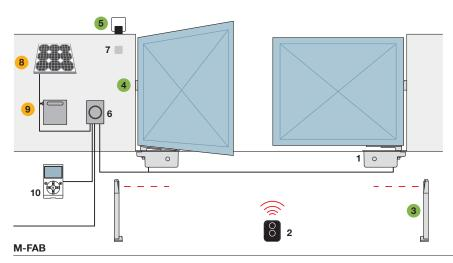
Motor 2. Transmitter 3. Photocells mounted on posts 4. Photocells 5. Flashing light 6. Control unit 7. Digital or key switch 8. SYP solar panel 9. PSY24 battery box 10. O-View multifunction display
