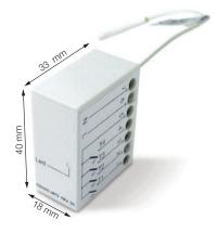
Recessed transmitters ideal for controlling automations not reachable directly by cable.
