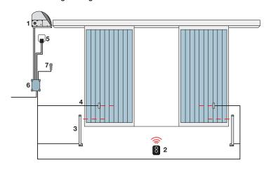
1. Motor 2. Transmitter 3. Photocells mounted on posts 4. Photocells 5. Flashing light 6. Control unit 7. Digital or key switches
