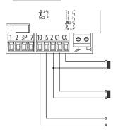
Photocells connection (NC contact), see the functions programming section.
