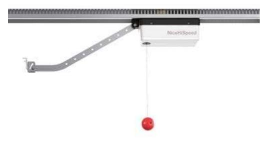
Electromechanical gearmotor, non-reversible, 24 VDC for residential use, rack-on-track drive. For use with SPYRAIL321, SPYRAIL162 and SPYRAIL081 tracks.
